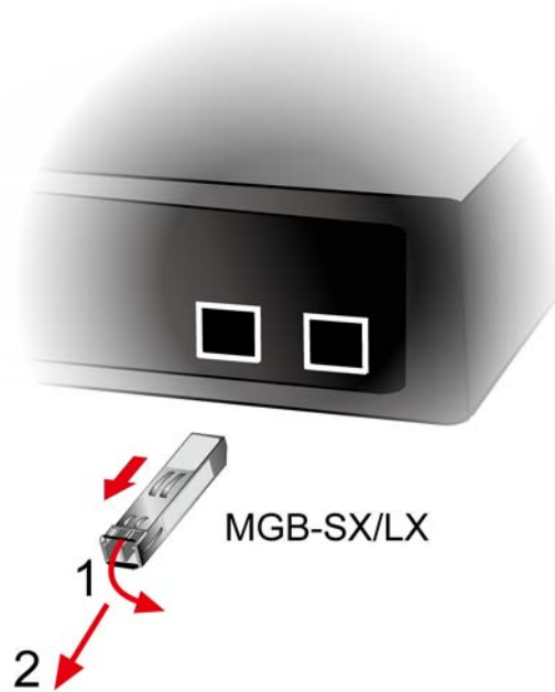
Figure 2-2-5: How to Pull Out the SFP / SFP+ Transceiver
