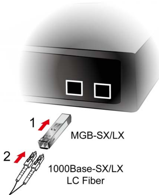
Figure 2-2-4: Plug-in the SFP/SFP+ Transceiver
